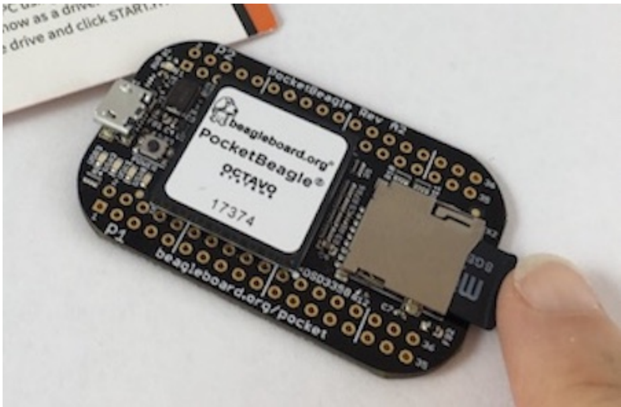
Fig. 3.10: Insert the microSD Card into PocketBeagle
