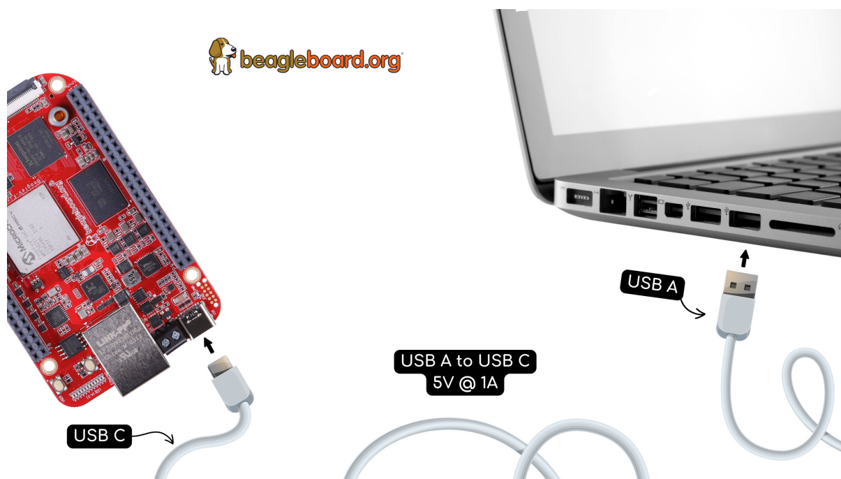
Fig. 2.2: BeagleV-Fire tethered connection
