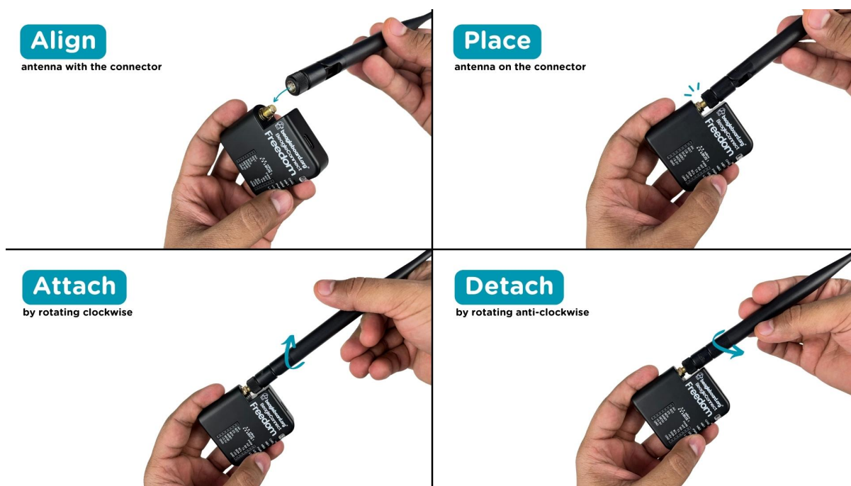
Fig. 2.2: Attaching antenna to BeagleConnect Freedom
